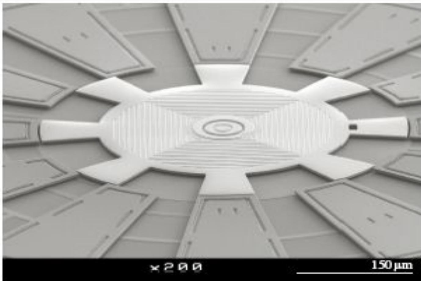
**Fig. 7.2** SEM micrograph of a surface-micromachined polysilicon micromotor fabricated using a SiO<sub>2</sub> sacrificial layer
