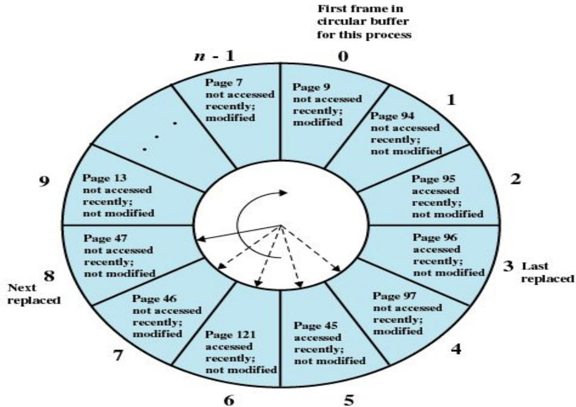
Figure 8.18 The Clock Page-Replacement Algorithm [GOLD89]
