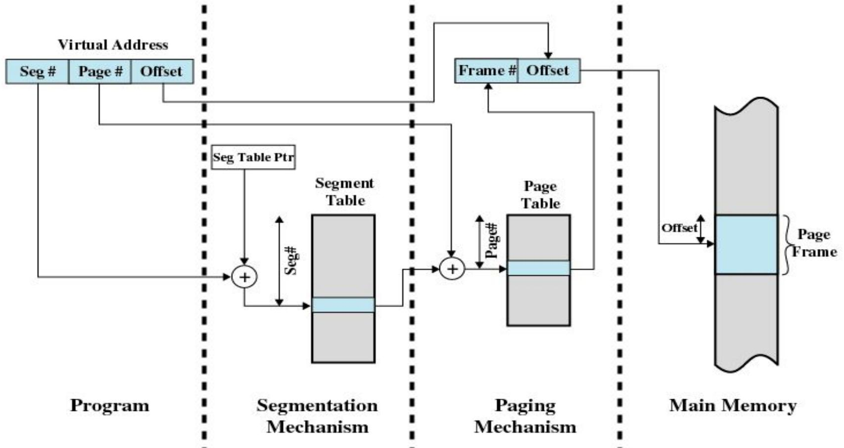
Figure 8.13 Address Translation in a Segmentation/Paging System
