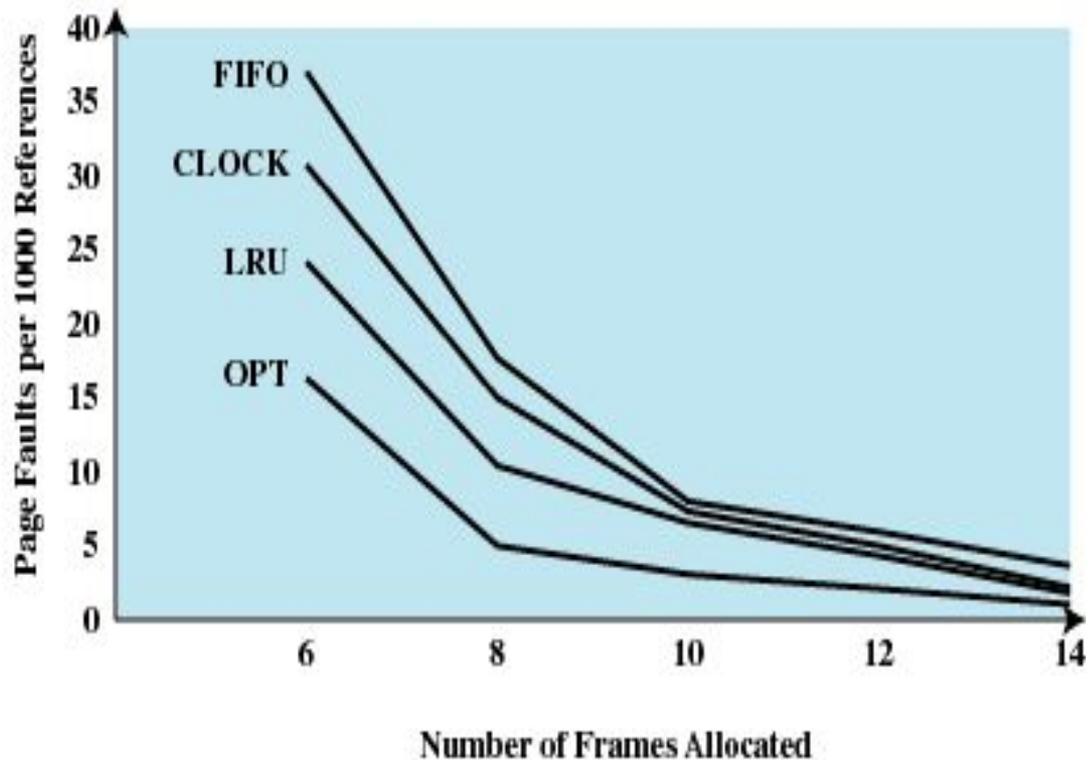
Figure 8.17 Comparison of Fixed-Allocation, Local Page Replacement Algorithms
