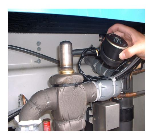
Step 3-2 Contact the Emergency magnet to the mounting of coil and open SMV fully by circulating of magnet
