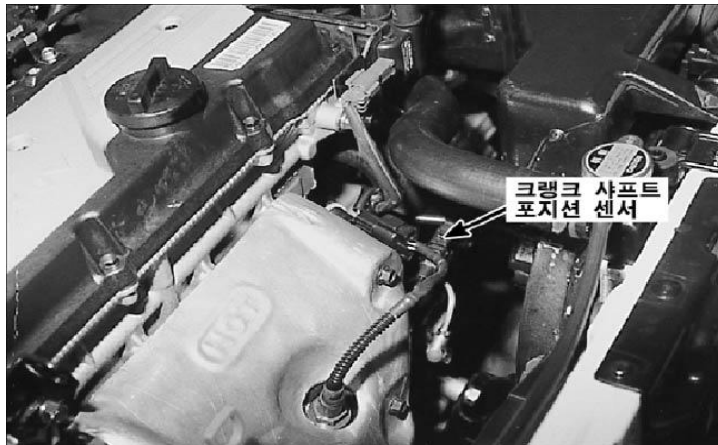
(a) DOHC Engine : LC, XD
