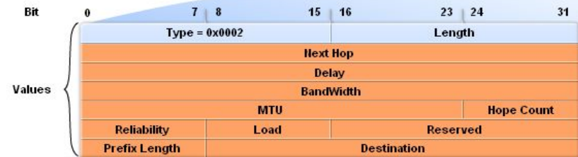
Type/Length/Values Types: IP Internal Routes TLV
