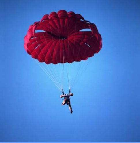
Parachute jumping as a sport began in the 1960s when new "sport parachutes" were first designed. The parachute above drive slots for greater stability and horizontal speed.
