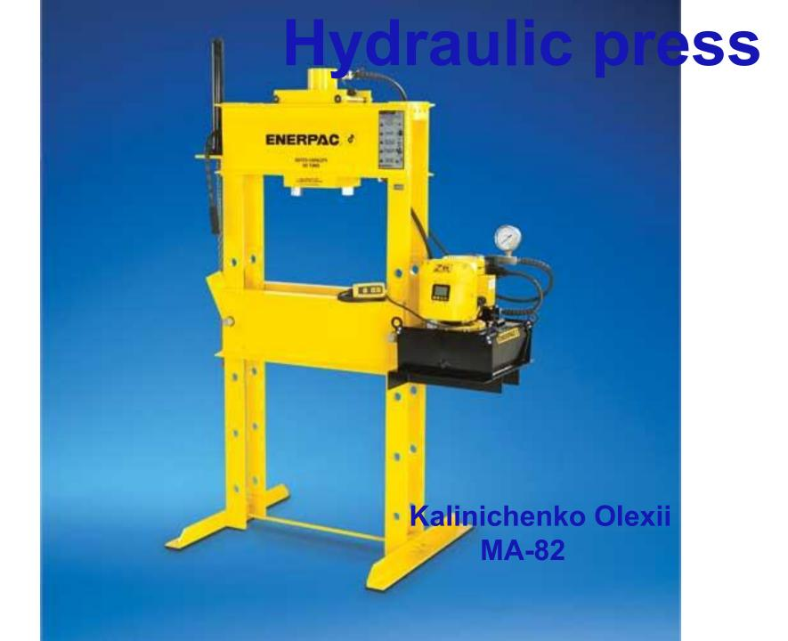
A hydraulic is a machine (see machine press) using a hydraulic cylinder to generate a compressive force. It uses the hydraulic equivalenta mechanical lever, and was also known as a Bramah press after the inventor, Joseph Bramah, of England. He invented and was issued a patent on this press in 1795. As Bramah (who is also known for his development of the flush toilet) installed toilets, he studied the existing literature on the motion of fluids and
