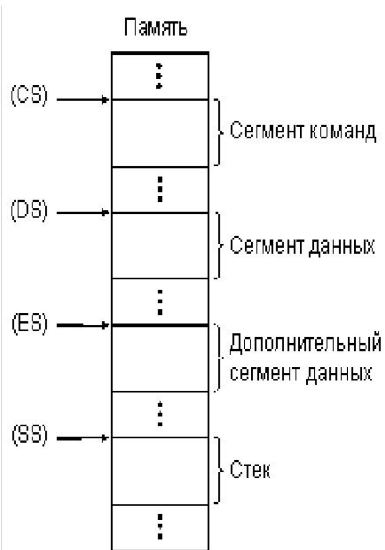
Fig. 1.5.10. Segments of commands, data and a stack in memory.
