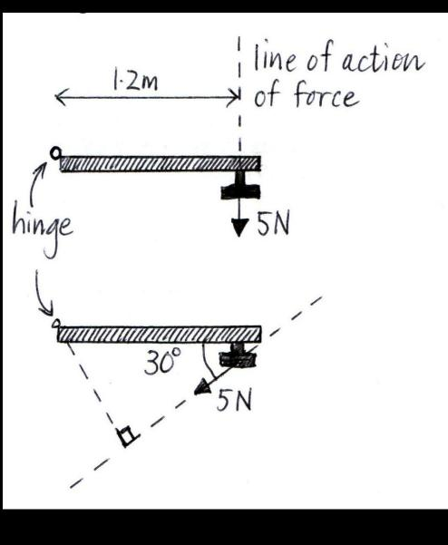
Principle of moments The principle of moments states that for a body to be in equilibrium: The sum of the external torques on a rigid object must be equal to zero
