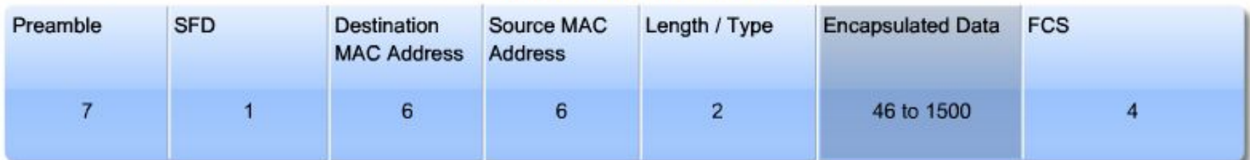
Structure of the Ethernet Frame
