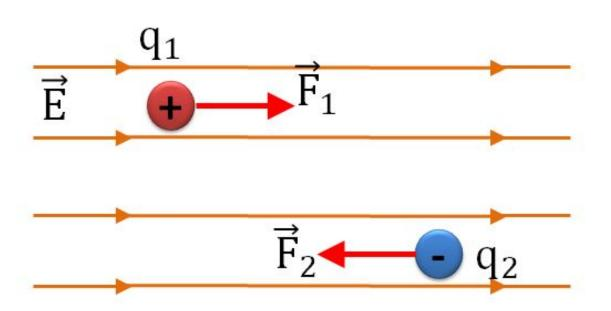
If we place a negatively and a positively charged particle in a uniform electric field, they experience forces in opposite directions.
