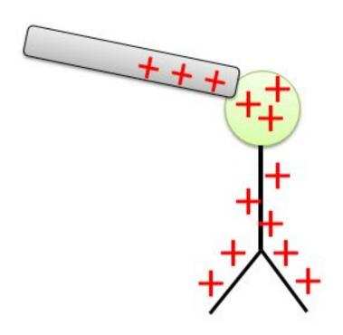
When the object touches the knob, the electroscope is charged positively. If we remove the object, the leaves remain separated. In both cases, the separation of the leaves is greater as the charge on the leaves is greater.
