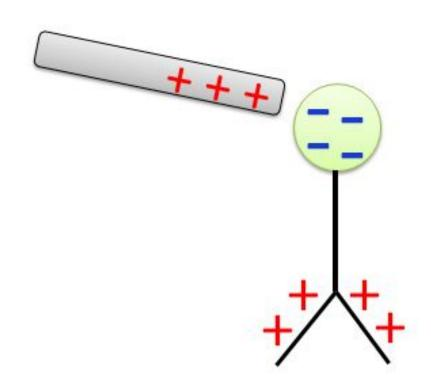
When a positively charged object is brought close to the knob, the leaves separate due to the free electrons which are attracted to the knob, thus the leaves both acquire the same amount of positive charge.
