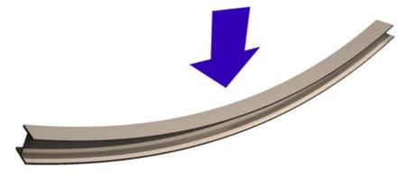
When vertical members can no longer resist a load they either *crush* or *buckle* (bending out of shape)
