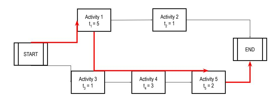
All inputs to an activity box must have been completed before it can begin.
