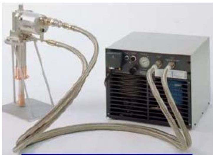
Used to build the first 4-K cryocooled superconductor product: Primary Voltage Standard
