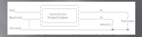
How do you monitor a line isolation transformer to see if there is any connection between both wire and ground?
