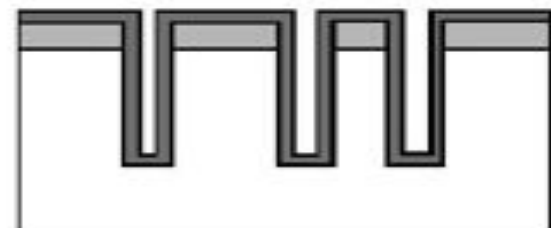
4. Coat sidewalls with PECVD oxide
