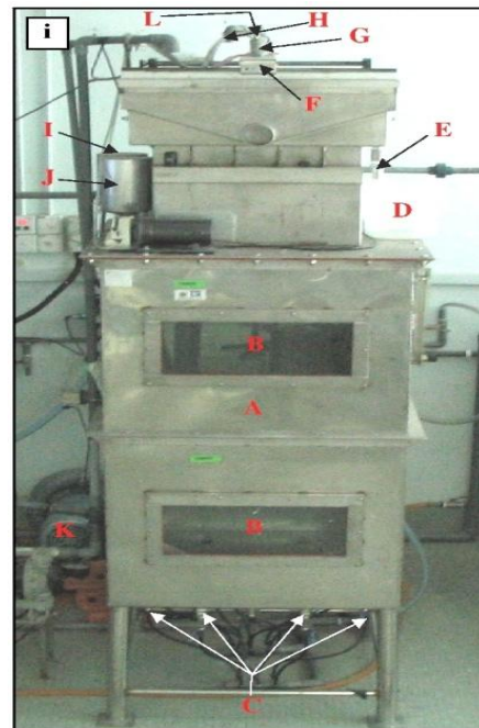
Flotation vessel; Front view (i) and Top view (ii). Note: A: Flotation vessel; B: Viewing glass; C: Nozzles; D: Ink reservoir; E: Foam outlet; F: Scraper; G: pH Probe; H: Thermocouple; I: acid/base reservoir; J: surfactant reservoir; K: Blower; L: water level sensor.
