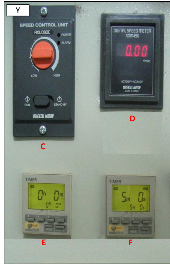
Mixing system provided in FERMSOSTAT®. (X) Speed control motor, (Y) Various digital readouts and (Z) Impeller.
