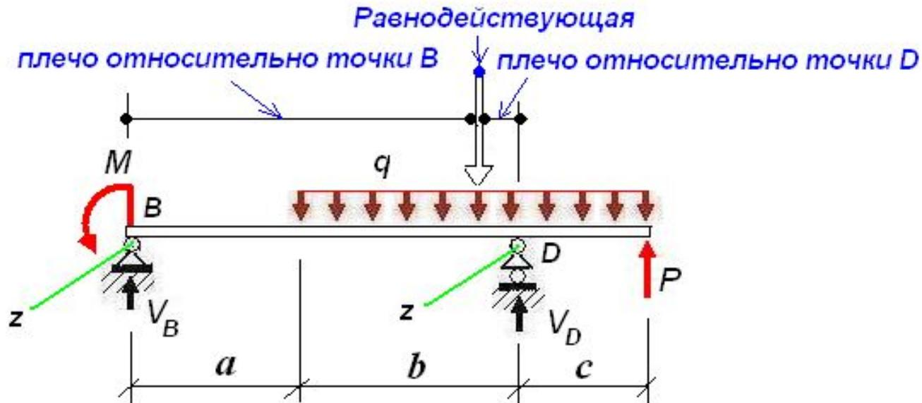
$$1. \sum m_B = V_D(a+b) + P(a+b+c) + M - q(b+c)\left(a + \frac{b+c}{2}\right) = 0 \Rightarrow V_D = \dots$$
