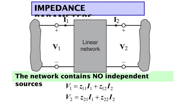
The '*z parameters*' can be derived in a manner similar to the Y parameters
