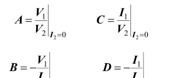
A = open circuit voltage ratio  $B = -\frac{V_1}{I_2}\Big|_{V_2=0}$  B = negative short - circuit transfer imperiate $<math display="block">B = -\frac{V_1}{I_2}\Big|_{V_2=0}$   $D = -\frac{I_1}{I_2}\Big|_{V_2=0}$  D = negative short - circuit current ratioB = negative short - circuit transfer impedance
