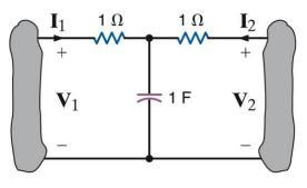
By splitting the 2-Ohm resistor, the network can be viewed as the cascade connection of two identical
