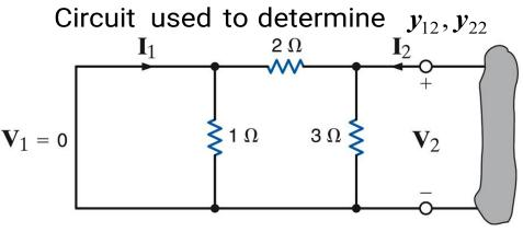
$I_{2} = \left(\frac{1}{2} + \frac{1}{3}\right)V_{2} \Rightarrow y_{22} = \frac{5}{6}[S]$  $-I_{1} = \frac{3}{2+3}I_{2} = \frac{3\times5}{5\times6}V_{2} \Rightarrow y_{12} = \frac{1}{2}[S]$
