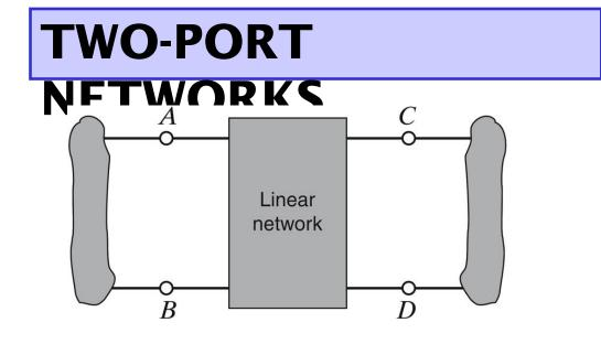
In many situations one is not interested in the internal organization of a network. A description relating input and output variables may be sufficient
