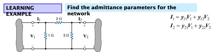
Circuit used to determine  $y_{11}, y_{21}$
