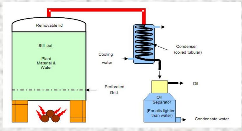
Diagrammatic representation of a steam and water distillation unit with a baffle to prevent direct water contact with the plant material on the perforated grid.
