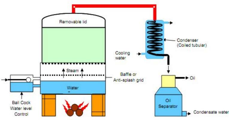
**Steam distillation** is the process of distilling plant material with the steam generated outside the still in a stand-alone boiler.
