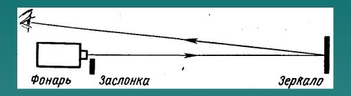
The figure shows a diagram of the experience through which Galileo proposed to measure the speed of light. Opening the valve lantern, you need to determine how to return the light reflects from the mirror.
