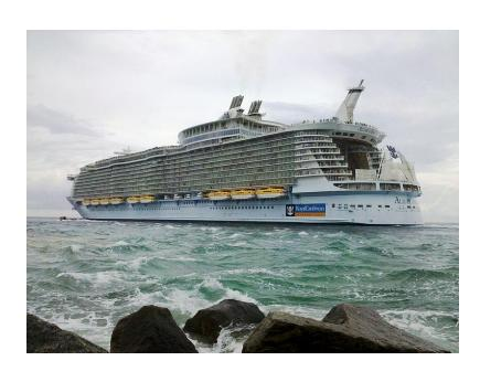
The <u>gross tonnage</u> of theAllure is 225,282 and her displacement — the actual weight of the ship — is equal to that of the Oasis, which is estimated to be around 100,000 metric tons, slightly less than that of an American Nimitz-class aircraft carrier. Her steel hull alone weighs roughly 54,000 tons.
