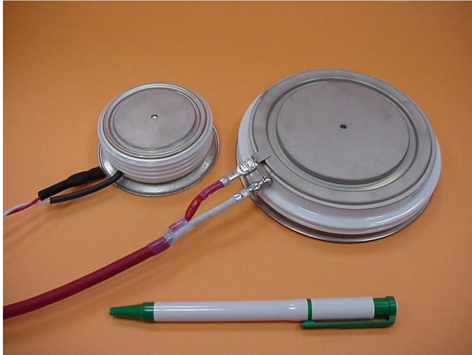
4500V/800A and 4500V/1500A SCRs
