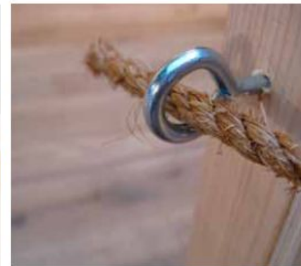
Thread the rope through the eyebolt
