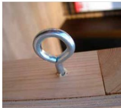
Screw in the eyebolts to the top corners of the wood panels
