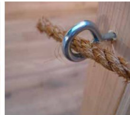
Thread the rope through the eyebolt
