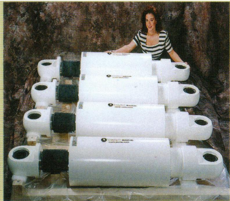
Passive Energy Dissipators for the Sidney Lanier Bridge, Georgia, USA. The bridge utilizes Taylor Dampers to control earthquake response, to reduce and distribute seismic loads while allowing free thermal movement.
