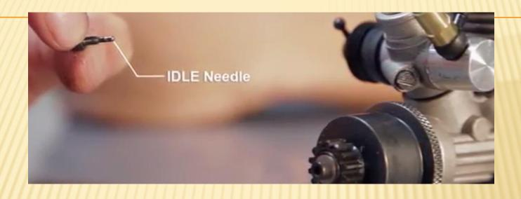
Idle needle regulates the carb opening and acts like a stop of the carb whenever you break.
