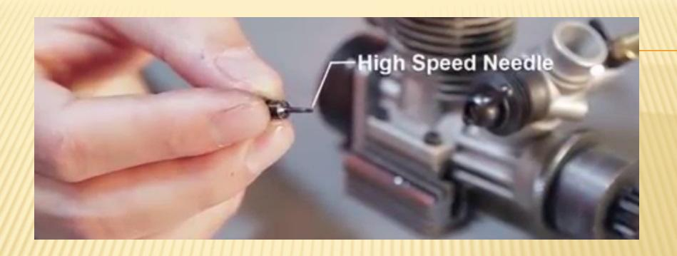
**High speed needle** regulates the entry of fuel to the engine in middle to high rpm.
