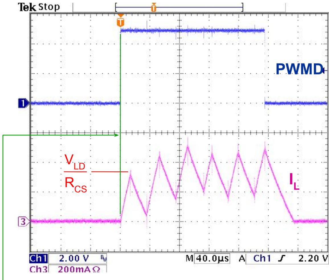
При ШИМ димировании, there is no delay. Auto\_ref= $V_{LD}$  initialized during PWMD=0.
