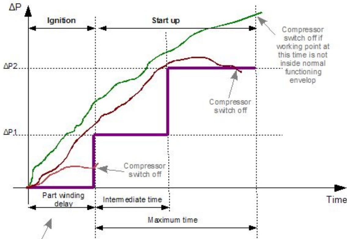
During this phase  $\Delta P$  isn't checked, the duration depends on compressor timing
