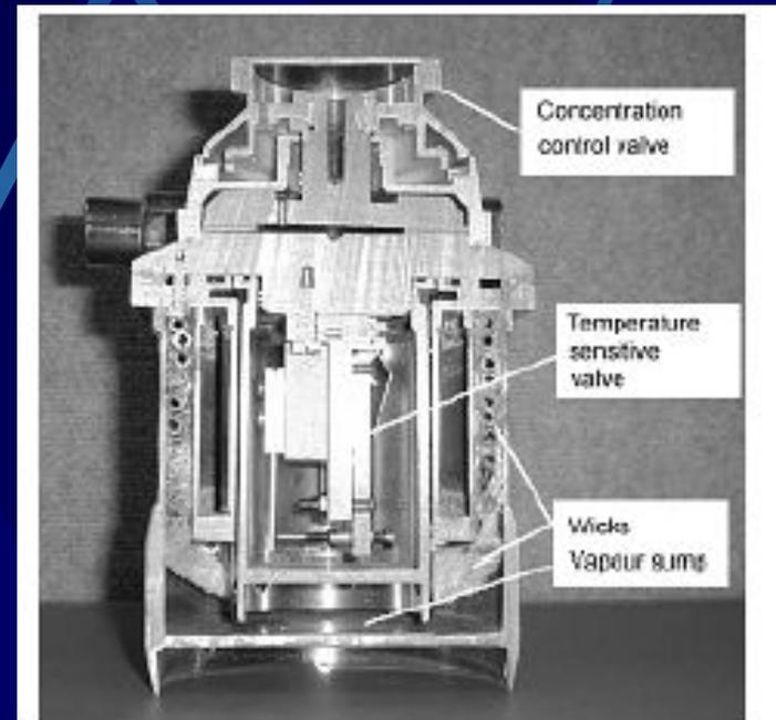
*Figure 2b: Cut-away view of a Fluotec2 halothane vaporiser (Cyprane, UK) Note the solid metal structure which acts as a heat sink and the wicks to aid vaporisation. Note the complex internal construction of the temperature compensation valve which causes high internal resistance in contrast to the EMO (figure 3a). This vaporiser cannot be used in a drawover mode.*
