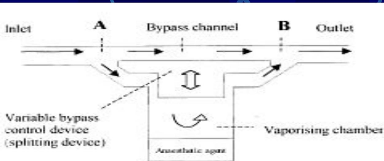
*Figure 1: Basic elements of a vaporiser:*
