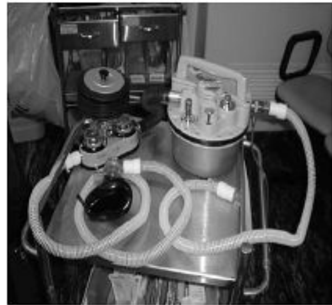
Figure 3a: The EMO ether vaporiser. Note the mass of water providing the heat sink, and the temperature compensation device - an ether filled bellows
