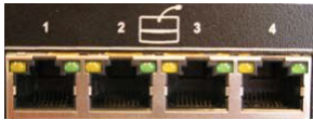
2. 4 x RJ45 ports to connect up to max 50 delegate units. (max. 25 units per branch or loop)
