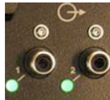
Two unbalanced RCA audio output connectors to extract analog audio floor signal Figure 7.6 : Aux Out The green indicators light up when there is an output signal > -40dBV present
