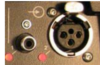
Two unbalanced RCA audio output connectors to extract analog audio floor signal Figure 7.6 : Aux Out The green indicators light up when there is an output signal > -40dBV present
