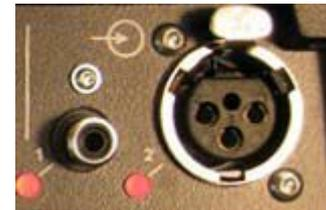
6. One unbalanced RCA analog audio input connector to add external signal to the floor
