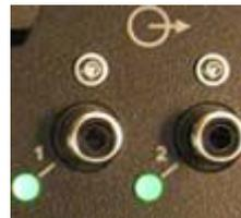
Two unbalanced RCA audio output connectors to extract analog audio floor signal
