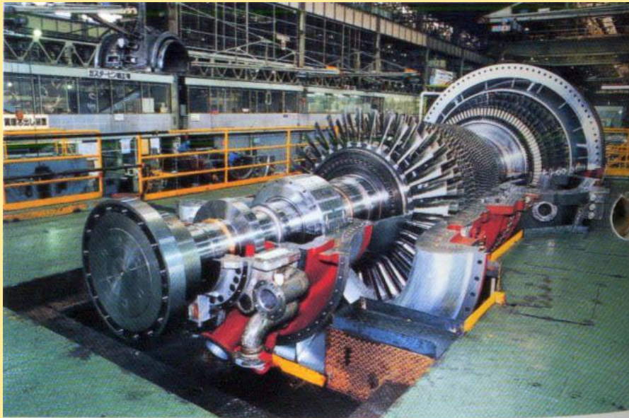
130 MW class Low BTU Gas Firing Turbine (M701D)
