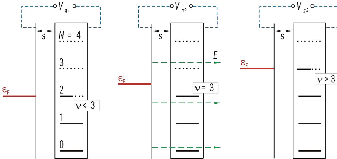
$$\Delta^{(i)} V_g = \frac{\hbar \Omega}{e} = \frac{\hbar B}{m c}$$
