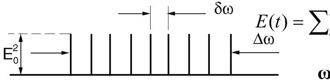
$$E(t) = \sum_{l=-n}^n E_0 \exp\{i[(\omega_0 + l\Delta\omega)t + l\varphi]\}$$
