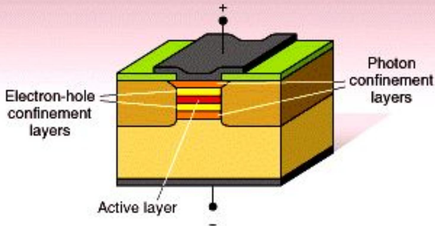
Quantum-well structure of an early gallium indium phosphide visible-output laser diode includes an active layer of less than 20-nm thickness (the layers are not drawn to scale). Aluminum was mixed with gallium indium to form the confining layers.
