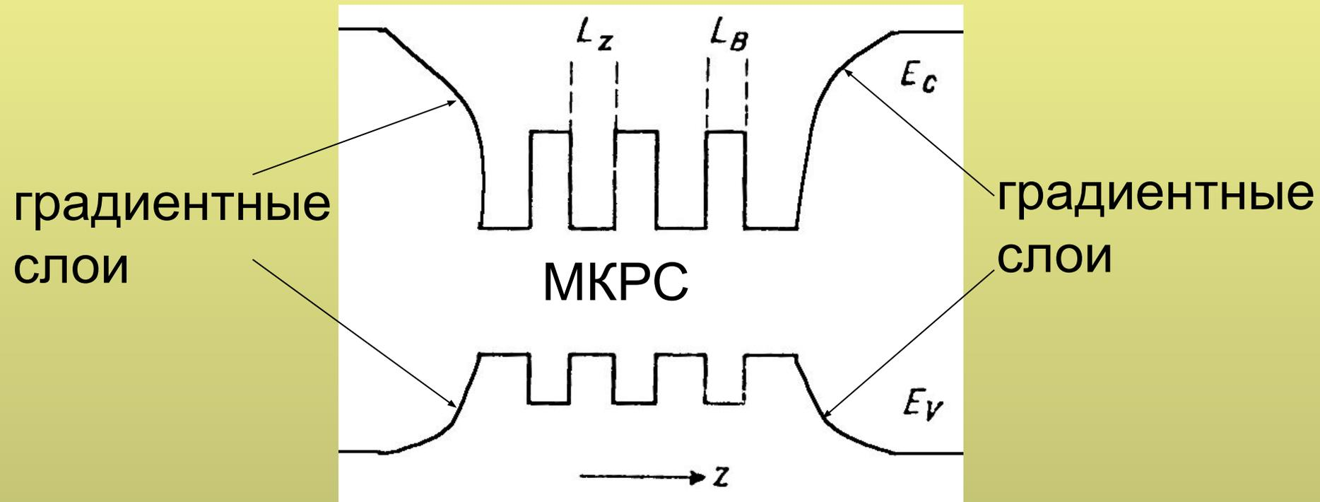
graded-index separated confinement heterostructure
