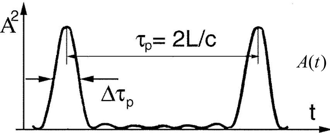
$$A(t) = E_0 \frac{\sin[(2n-1)(\Delta\omega t + \varphi)/2]}{\sin[(\Delta\omega t + \varphi)/2]}$$
