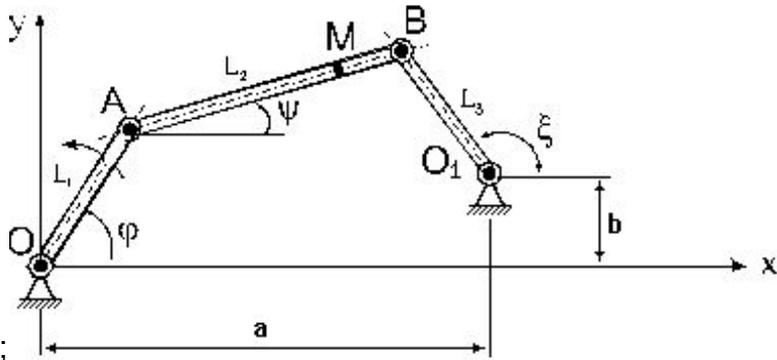
$$\begin{aligned} a - L_1 \cos \varphi &= L_2 \cos \psi - L_3 \cos \xi; \\ b - L_1 \sin \varphi &= L_2 \sin \psi - L_3 \sin \xi. \end{aligned} \quad (\text{a})$$
