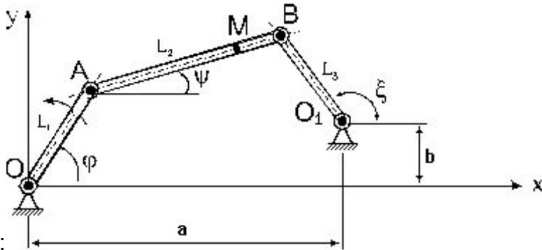
$$\begin{aligned} a - L_1 \cos \varphi &= L_2 \cos \psi - L_3 \cos \xi; \\ b - L_1 \sin \varphi &= L_2 \sin \psi - L_3 \sin \xi. \end{aligned} \quad (a)$$
