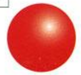
Diameter 0.5 mm Uranium dioxide Fuel
