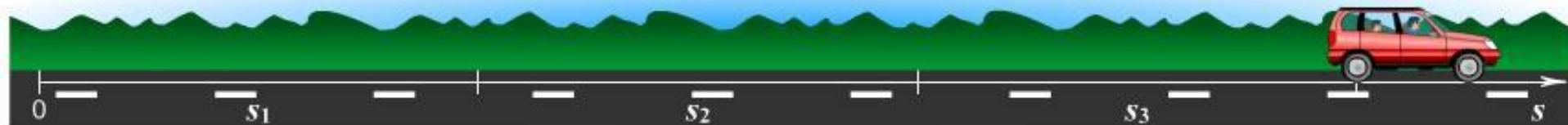
$$v_{\text{cp}} = \frac{s_1 + s_2 + s_3}{t_1 + t_2 + t_3}$$
