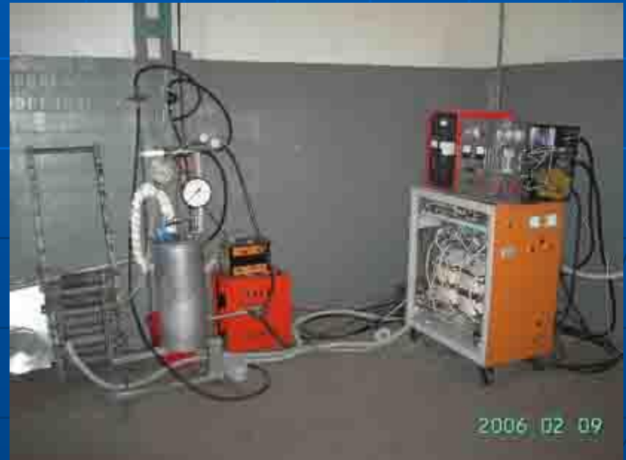
Laboratory Steam Plasma Machine by capacity of 40 KW
