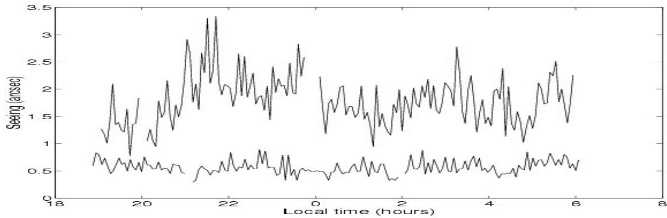
**Maidanak seeing measured by DIMM in arcseconds at zenith and 0.5  $\mu$ m: examples of a good and a bad nights**
