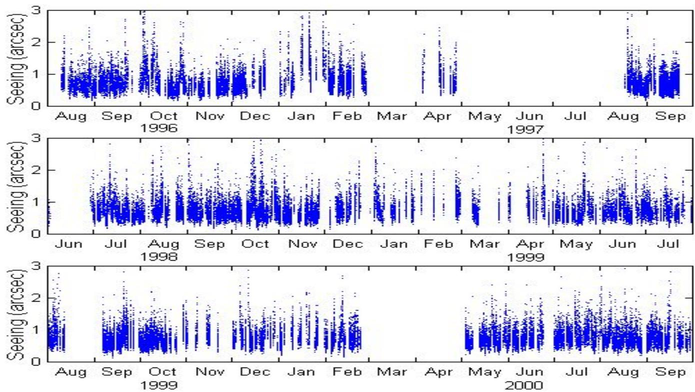
**The full series of seeing measurements obtained at Maidanak with the DIMM from August 1996 up to November 2000**
