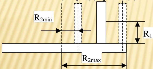
$$i_{\max} = \frac{\omega_1}{\omega_{2\min}} = \frac{n_1}{n_{2\min}} = \frac{R_{2\max}}{R_1 \cdot \zeta} \quad i_{\min} = \frac{\omega_1}{\omega_{2\max}} = \frac{n_1}{n_{2\max}} = \frac{R_{2\min}}{R_1 \cdot \zeta}$$
