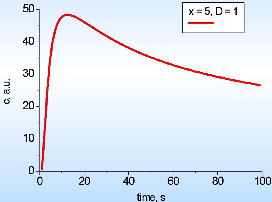
$$\frac{\partial c}{\partial t} = \frac{N}{\sqrt{4\pi Dt}} \exp\left(-\frac{x^2}{4Dt}\right) \left(-\frac{1}{2t} + \frac{x^2}{4Dt^2}\right)$$
