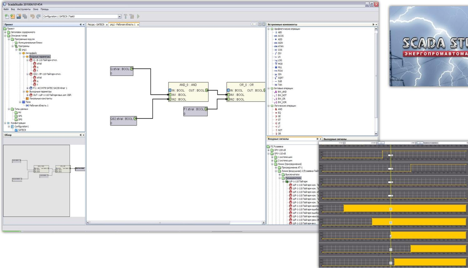
The screenshot displays the SCADA NPT Expert software interface. The main window shows a logic diagram with several input variables (D.stval, OS2.stval, F1.stval) connected to an AND gate (AND\_0) and an OR gate (OR\_0). The AND gate has two inputs (IN1, IN2) and one output (OUT). The OR gate has two inputs (IN1, IN2) and one output (OUT). The output of the AND gate is connected to the input of the OR gate. The output of the OR gate is connected to a signal output.
