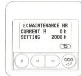
Planned maintenance hour meter
