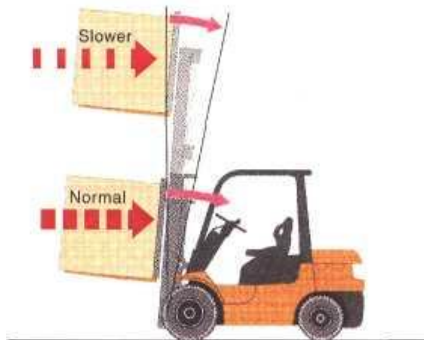
SAS Mast Rear Tilt Speed Control
