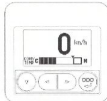
Digital speedometer, transmission oil temperature indicator
