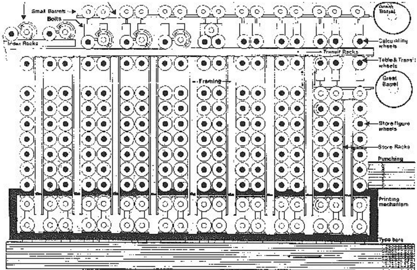
Fig. 2. Plan of Analytical Engine with grid layout, 1858. Redrawn.
