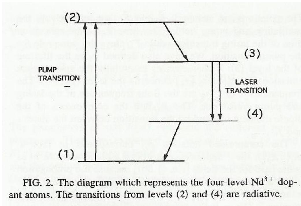
FIG. 2. The diagram which represents the four-level Nd<sup>3+</sup> dopant atoms. The transitions from levels (2) and (4) are radiative.
