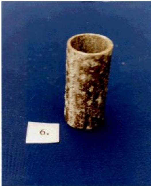
Changes caused by corrosion in both external and internal surface of magnesium tube No 7(311 /97)
