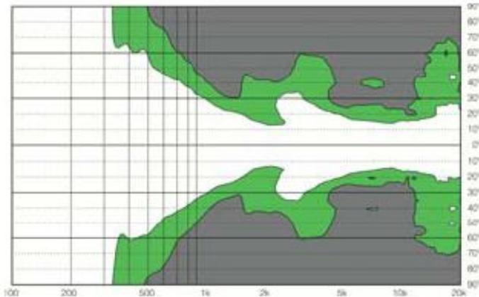
Dispersion of the Convert 15A with the DCD set at 40°
