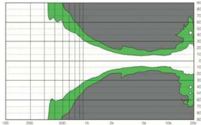
Dispersion of the Convert 15A with the DCD set at 20°
