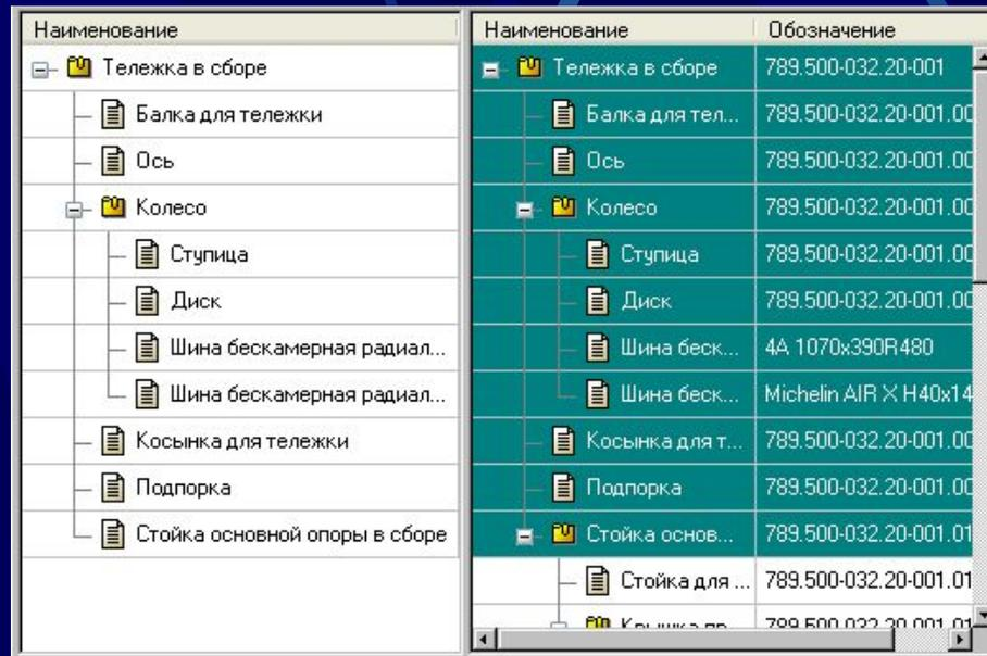
The screenshot displays a software interface with two main panels. The left panel shows a hierarchical tree structure of components, and the right panel shows a table of attributes for the selected components.
