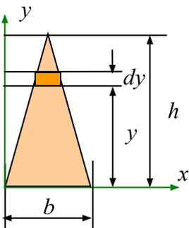
$$y_c = \frac{\int y dS}{\int dS} = \frac{\int_0^h y \frac{h-y}{h} b dy}{\int_0^h \frac{h-y}{h} b dy} = \frac{\frac{b}{h} \int_0^h (hy - y^2) dy}{\frac{b}{h} \int_0^h (h-y) dy} = \frac{\frac{b}{h} \left( h \frac{y^2}{2} - \frac{y^3}{3} \right) \Big|_0^h}{\frac{b}{h} \left( hy - \frac{y^2}{2} \right) \Big|_0^h} = \frac{\frac{bh^2}{6}}{\frac{1}{2} bh} = \frac{h}{3}$$
