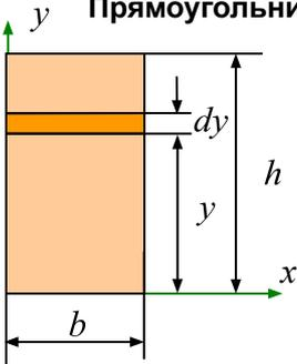
$$y_c = \frac{\int y dS}{\int dS} = \frac{\int_0^h y b dy}{\int_0^h b dy} = \frac{b \int_0^h y dy}{b \int_0^h dy} = \frac{b \frac{y^2}{2} \Big|_0^h}{bh} = \frac{h}{2}$$
