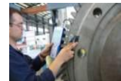
Dovetail EC inspection
