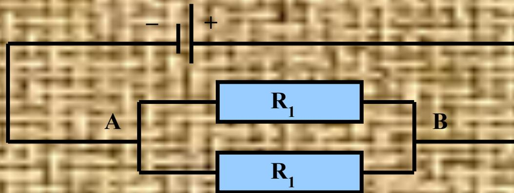
$$\frac{1}{R} = \frac{1}{R_1} + \frac{1}{R_2} = \frac{1}{R_1} + \frac{1}{R_1} = \frac{2}{R_1},$$
